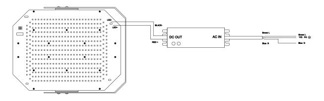
Remove or bypass the ballast, capacitor and ignitor.
